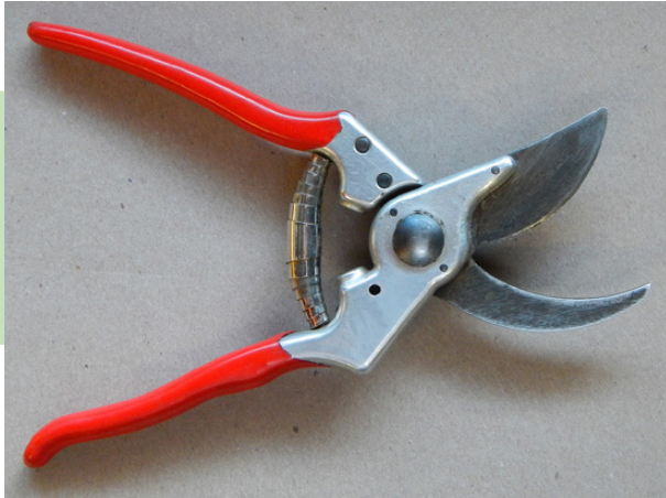
Above: Clippers with a wrapped metal spring. These are fantastic clippers, I have to take the spring off and clean it occasionally.
