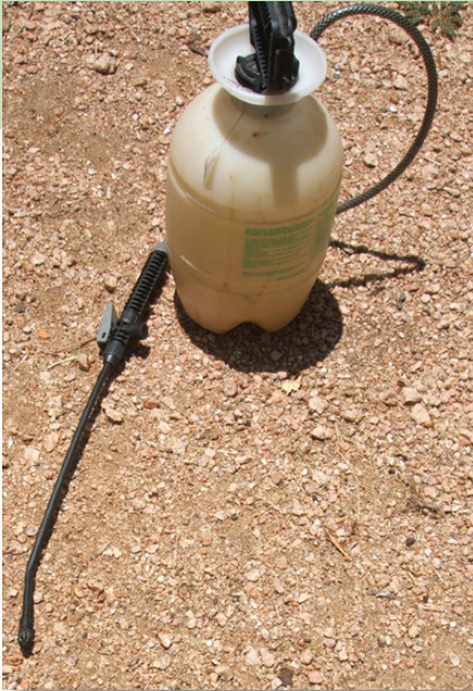
Hand-pump sprayer, used here to apply a solution of horticultural vinegar on weeds in gravel areas.
