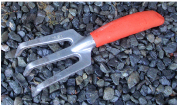
Above: a good claw tool, notice the metal is all one piece with rubber wrapped around the handle for comfort.
