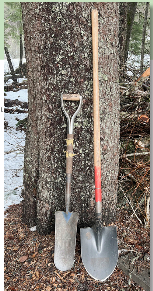
Above left is a sharp shooter, right is the standard spade shovel.
